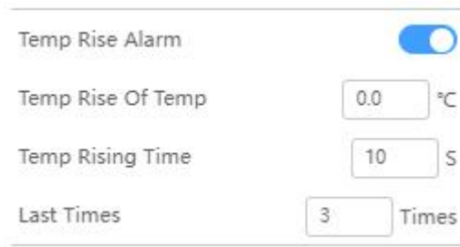
Figure 3.8 Measurement List-Temperature Rise Alarm Settings
