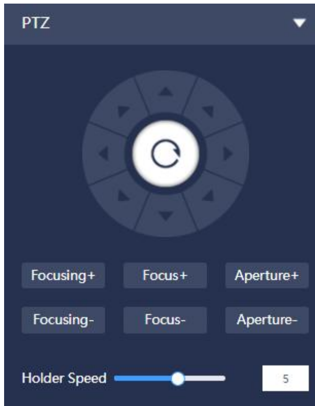
Figure 2.3 PTZ Control Interface
