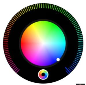
4. To make the light color temperature warmer or cooler, tap , and rotate the knob to adjust the slider.
