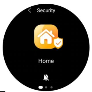
To enable the siren, tap , and enter the preset code. The icon turns to be indicating that the siren function is on.
